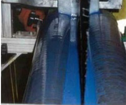
Fig: - Saturation of Carbon Fiber
